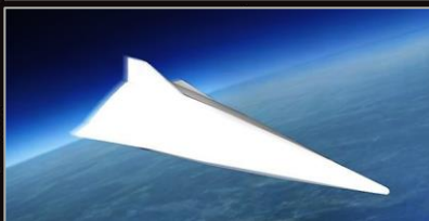
Figure 1: China's DF-ZF Hypersonic Glide Vehicle, capable of flying at speeds of between Mach 5 and Mach 10. [1]
